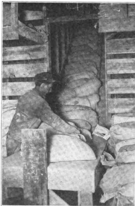
This chute delivers sacked materials from the cars on elevated tracks to the storage room on the second floor of the warehouse. From here materials are chuted thru trap doors to a loading platform on the ground floor, as shown in the illustration on the next page
